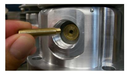
Thoroughly clean the base of the test tap cavity with isopropyl alcohol or acetone using a clean lint-free towel, focusing on the circular band of grey insulation (tap insulation) surrounding the tap contact plate. A thin band of white material (flange adhesive) may also be seen surrounding the band of grey insulation.
