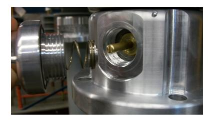
• Unscrew the test tap pin using a flat-head screwdriver.
