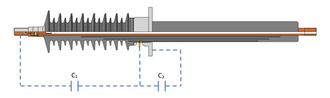
While the  $C_1$  layer is completely comprised of the epoxy that makes up an SDC core, the  $C_2$  layer is composed of a small layer of the core epoxy and a thin layer of structural adhesive (used to bond the flange onto the core). It is normal that the  $C_2$  power factor differ from the  $C_1$  power factor.
